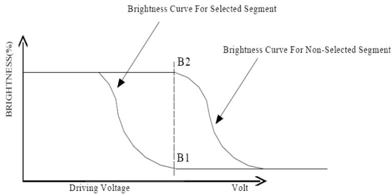
$$Cr = \frac{\text{Brightness of Non-selected Segment}(B2)}{\text{Brightness of selected Segment}(B1)}$$
